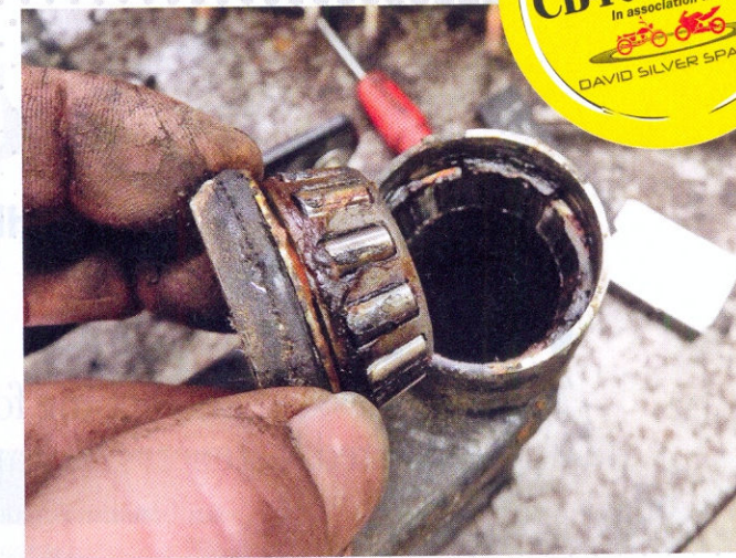
▶ Taper roller swingarm bearings are a bit of a mess and need replacing
